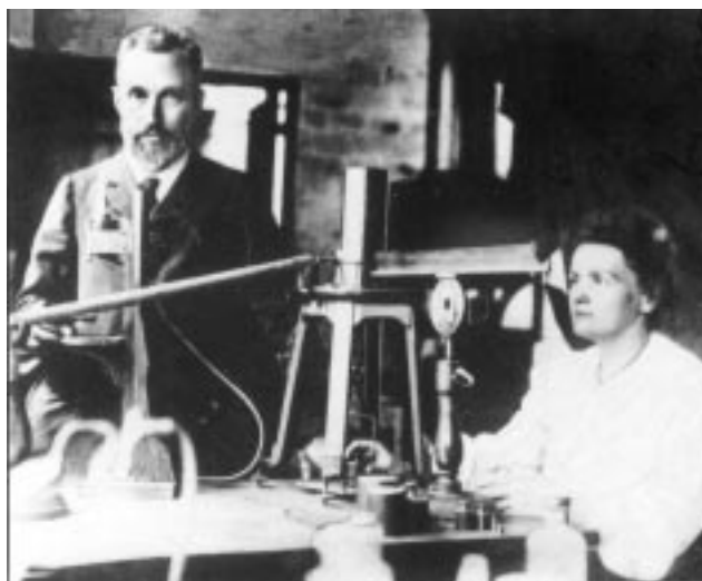
Fig. 5. Marie Curie proceeds to the measurement of a radioactive sample. With the right hand she lifts progressively the weight applied to the quartz; in the left hand she holds the chronometer.
